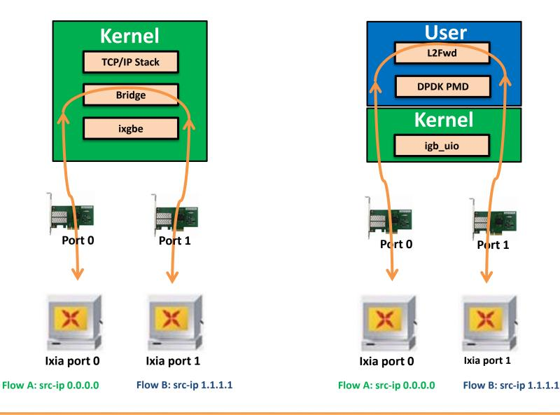
Aggregated Performance at 64B small packet : 1.35 Mpps vs. 23.68Mpps
